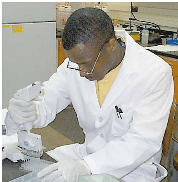
Figure 3. Adding reagents to a 96-well plate using a multichannel pipet
