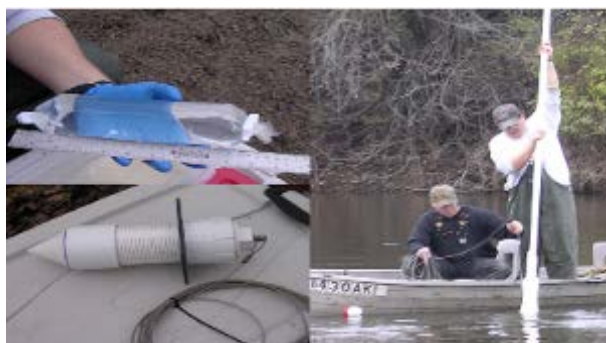
Peeper sampler (l), sampler installation (r).
