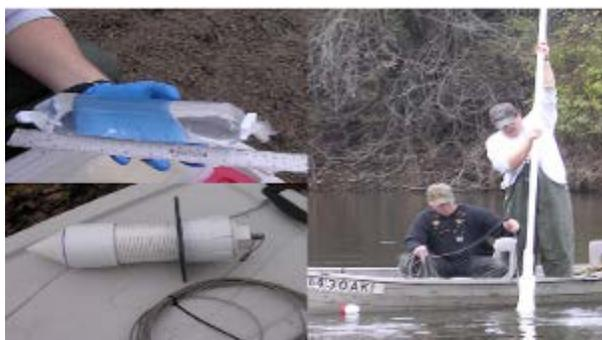
**Peeper sampler (l), sampler installation (r).**
