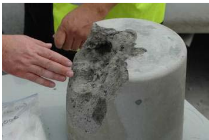
Figure 6-8. Five-gallon bucket-molded sample cleaved, exposing successful encapsulation of contaminant. Source: Portland Cement Association.
