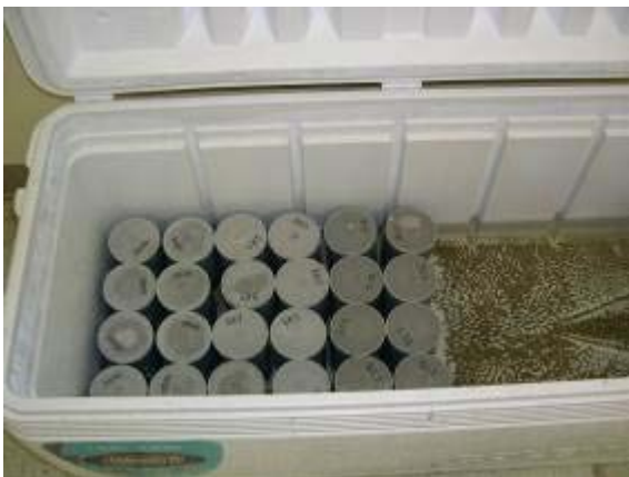
Figure 6-6. Field curing of S/S material specimens in a humid atmosphere (water bath). Source: Ed Bates.
