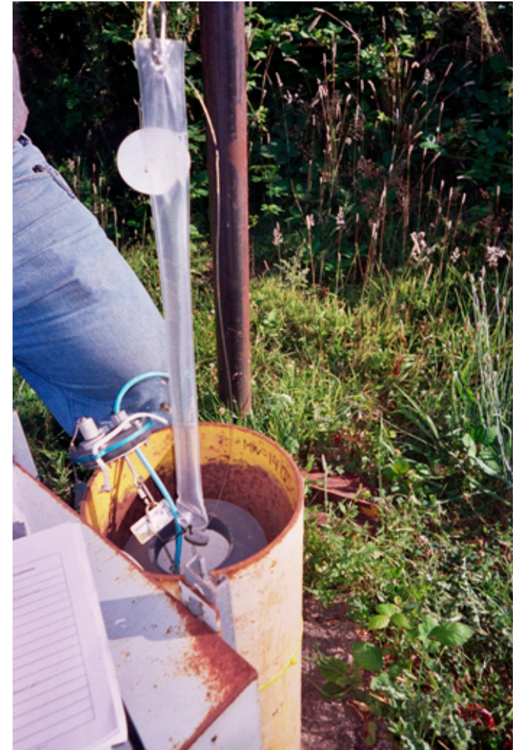
Passive diffusion sampler being placed in a monitoring well
