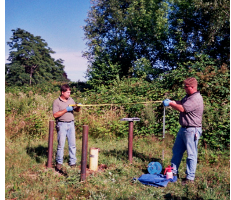
Installation of passive diffusion samplers at the East Multnomah County Cleanup Project
