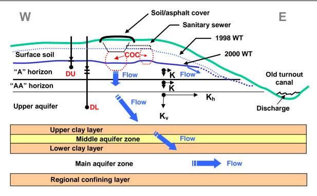
Figure 3-2. Revised conceptual site model suggesting a potential downward movement of contamination.
