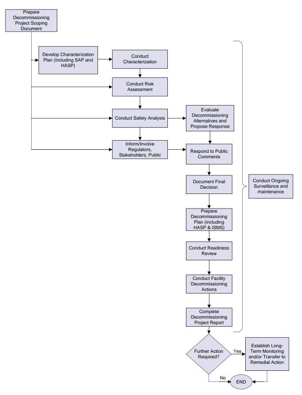
Figure 4-1. DOE decommissioning framework. Adapted from DOE 2000c.
