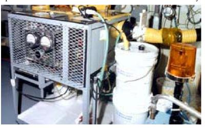
Figure 6-3. Use of the aerosol fogging equipment is intended to downgrade the personal protective equipment requirements for room entry from suppliedair suits to standard powered air-purifying respirators.
