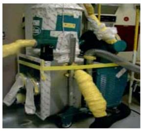
Figure 6-5. Raschig ring vacuum system.
