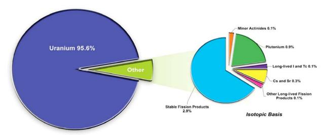
Figure 2-1. Approximate composition of spent fuel, based on DOE data. "Other" actinides include plutonium and minor actinides, and all remaining categories are included in fission products.
