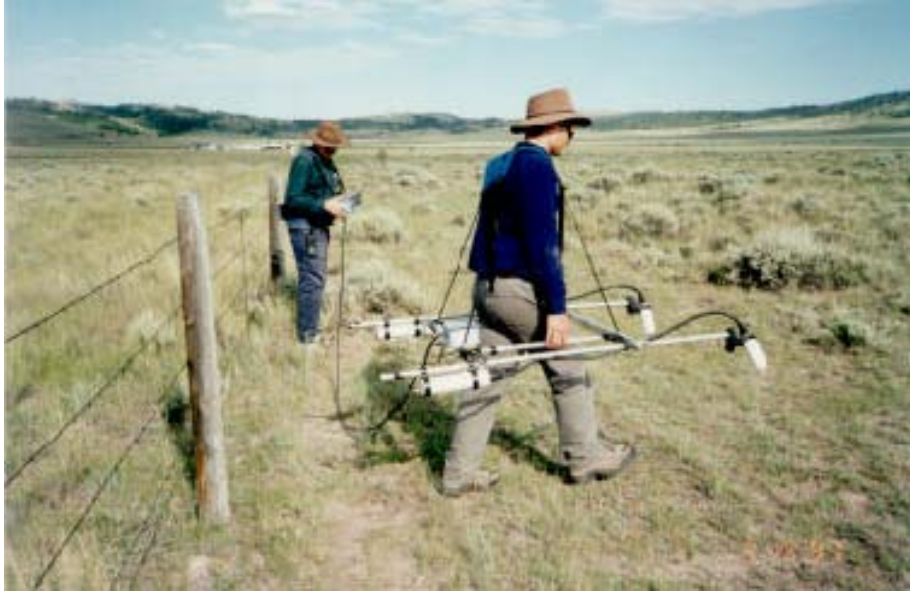
Figure 4-2. Man-portable, dual-sensor cesium-vapor magnetometer.
