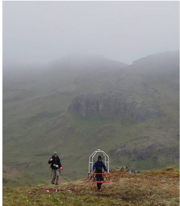
Operators performing a man-portable DGM survey during an MR project on Adak, Alaska.
